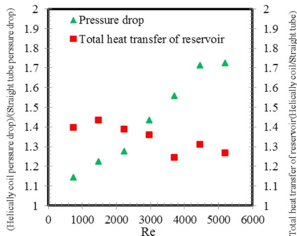
Figure 4. Comparing performance of coiled tube on heat transfer and pressure drop
