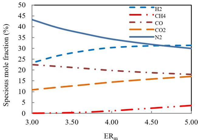
Figure 1. Biogas composition V.S.  $ER_m$
