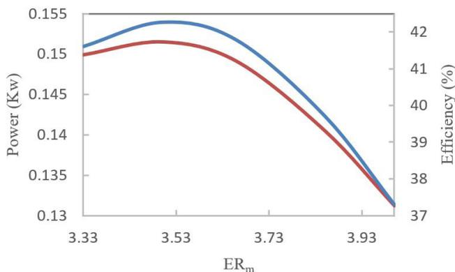
Figure 2. SOFC power and efficiency V.S.  $ER_m$
