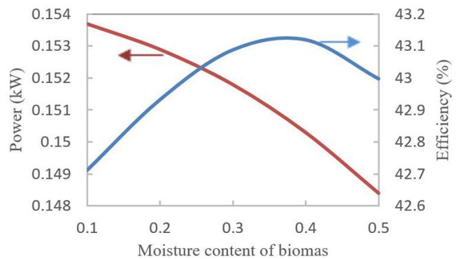
Figure 4. SOFC power and efficiency V.S. MC
