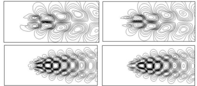
Figure 3. Streamwise velocity contour for missing data with 90% (left-top), original snapshot (right-top), reconstructed using simple iterative method (left-bottom) and reconstructed using time advancing iterative method (right-bottom)
