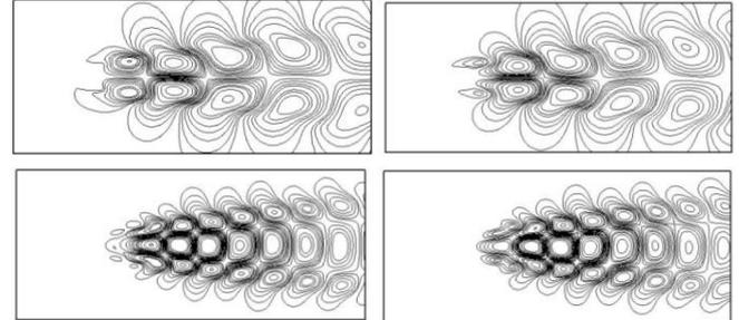
Figure 1. Four strongest modes of streamwise velocity component
