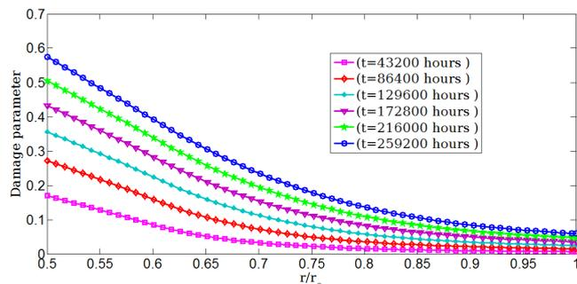
Figure 2. Changes in creep damage along the thickness of cylinder after (259200 hours) from the beginning of creep process.
