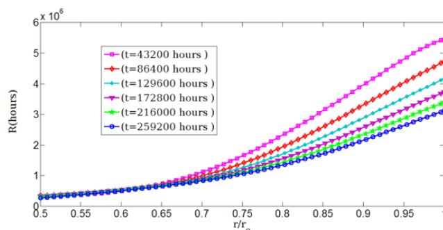
Figure 3. Remnant life histories of rotating hollow shaft from initial elastic up to 259200 hours.
