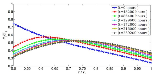
Figure 5. Dimensionless circumferential stress redistribution of rotating hollow shaft from its initial elastic up to 259200 hours.
