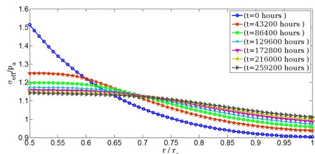
Figure 6. Dimensionless effective stress redistribution of rotating hollow shaft from its initial elastic up to 259200 hours.
