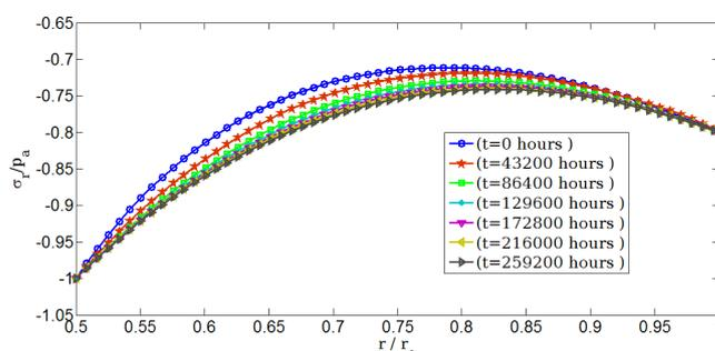
Figure 4. Dimensionless radial stress redistribution of rotating hollow shaft from its initial elastic up to 259200 hours.
