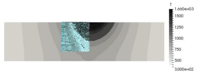
Figure 4. Comparison of calculated and experimental weld geometry at laser power of 1700 W, speed of 13.43 mm/s and depth of 0.5 mm
