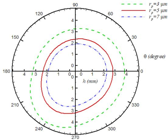
Figure 5. Effect of particle radius on the cake thickness
