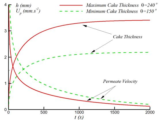
Figure 2. Rate of cake growth and permeate flux with time at maxima and minima of cake thickness
