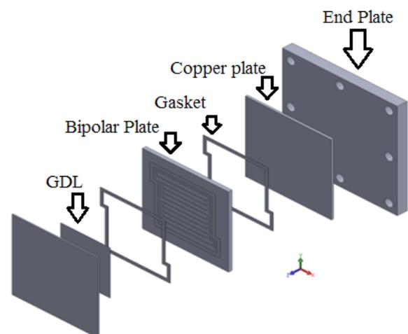
Figure 1. The employed single fuel cell stack model
