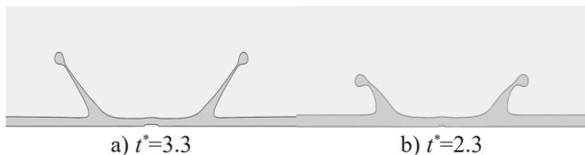
**Figure 3. A Droplet Splashing on a Thin Liquid Film in  $Re=240$  and  $We=800$  (Left),  $We=500$  (Right)**
