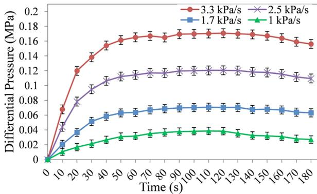
Fig. 4. The differential pressure versus time for  $P_i=3.5$  MPa and orifice diameter of 0.5 mm
