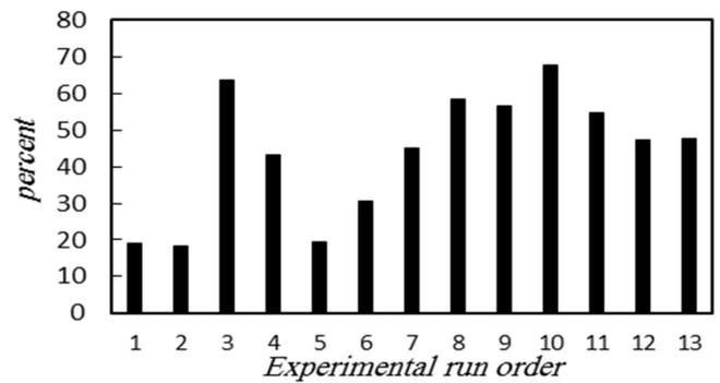
**Fig. 3. Percent of tool wear improvement in cryogenic status**
