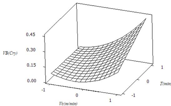
**Fig. 1. 3D surface graph for interaction effects of cutting time and cutting speed on the tool life in dry machining**
