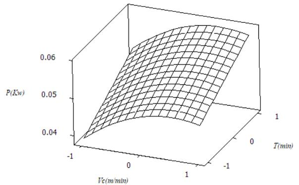
**Fig. 4. 3D surface graph for interaction effects of cutting time and cutting speed on power consumption in dry machining**
