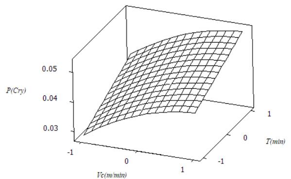
**Fig. 5. 3D surface graph for interaction effects of cutting time and cutting speed on power consumption in cryogenic machining**
