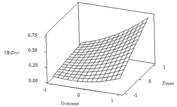
**Fig. 2. 3D surface graph for interaction effects of cutting time and cutting speed on tool life in cryogenic machining**
