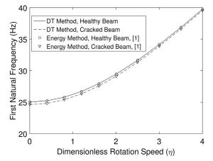
Fig. 2. Effect of the rotation speed on the fundamental natural frequency of a healthy and cracked beam
