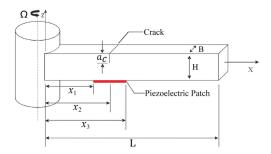
Fig. 1. A cracked rotating beam with a piezoelectric patch
