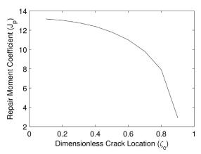
Fig. 3. Effect of the crack location on the repair moment coefficient
