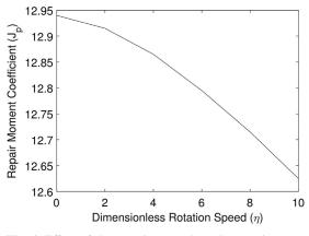
5- Fig. 4. Effect of the rotation speed on the repair moment coefficient
