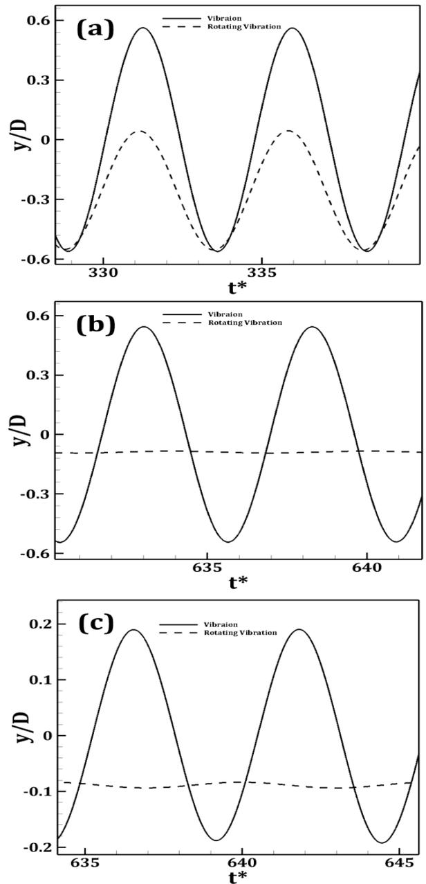
Fig. 3. Time histories of the cylinder displacement for a) the single cylinder, b) the front cylinder and c) the rear cylinder for two cylinders
