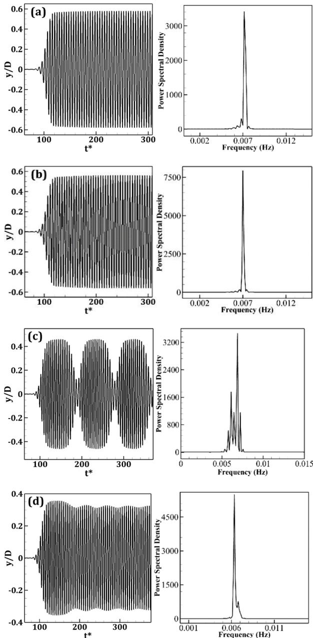
Fig. 2. Time histories of the cylinder displacement and FFT for the reduced velocity of 4 and the damping ratio of a) 0, b) 0.01, c) 0.05 and d) 0.1
