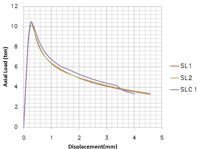
Fig. 7. FEM load-displacement curves
