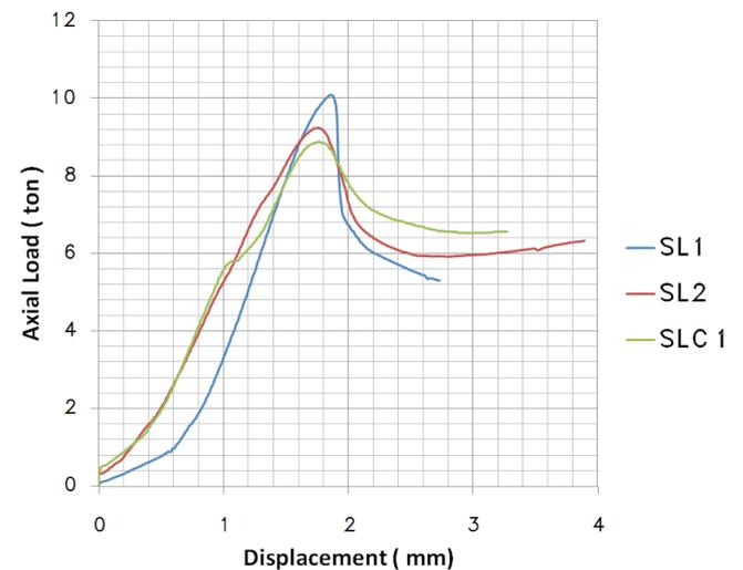
**Fig. 5. Experimental load-displacement curves**
