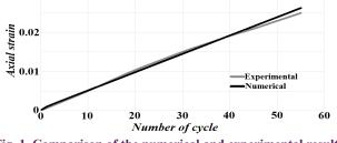
Fig. 1. Comparison of the numerical and experimental results for axial ratcheting on the intrados place.
