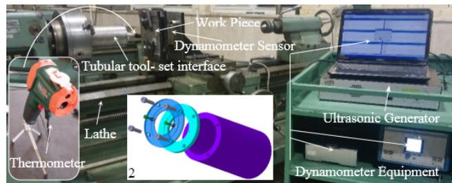
Fig. 3. 1- Experimental set up of UaFSW process, 2- Tubular interface between the toolset and the lathe chuck
