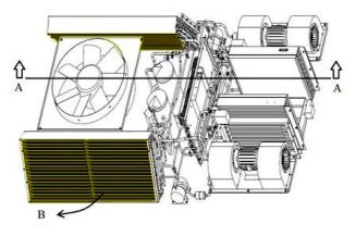
Fig. 1. View of air conditioning system in subway train
