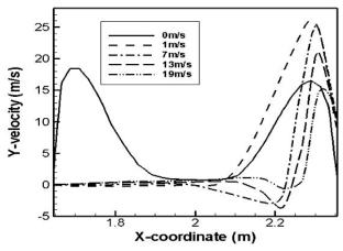
Fig. 4. Variation of vertical velocity over the subway train roof for different train speeds
