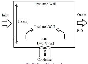
Fig. 2. View of the tunnel
