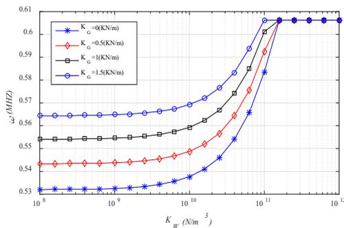
**Fig. 2. Effects of orthotropic elastic foundation on the natural frequencies of double-bonded micro plates**
