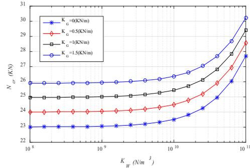
**Fig. 3. Effects of orthotropic elastic foundation on the critical buckling load of double-bonded micro plate**
