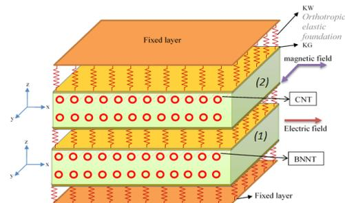
Fig. 1. Geometry of double-bonded micro composite plates reinforced by CNTs and BNNTs
