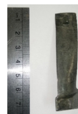
Fig. 1: Forged titanium blade after burr cutting.
