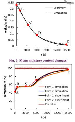
Fig. 4. Two surface points temperature changes
