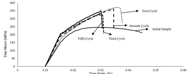
**Fig. 4: True stress-strain curves of ARB samples**
