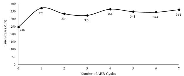
**Fig. 5: Tensile strength variations in ARB samples**
