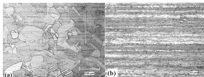
Fig. 1. The microstructure of brass and aluminum sheets used in ARB process (a) brass and (b) aluminum
