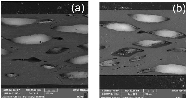
**Fig. 2: The cross-section of ARB samples in the rolling direction after (a) 5 and (b) 7 cycles**
