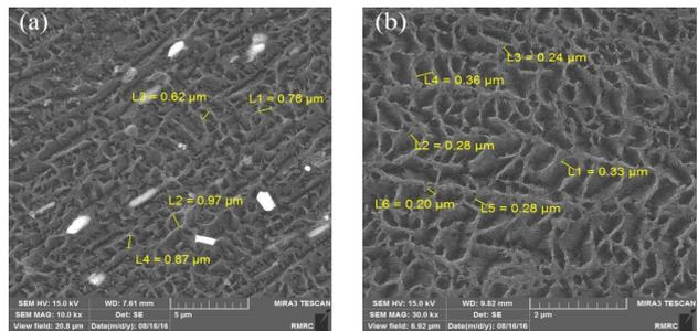
**Fig 3: The grain size of the ARB sample after (a) 5 and (b) 7 cycles**
