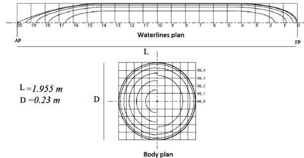
Fig. 1. Dimensions and the body lines of the Joubert submarine model [3]
