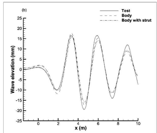
Fig. 4. Free surface changes observed in the test, model analysis and model analysis with the strut at speed of 2.19 m/s and  $D^* 2.2$ .
