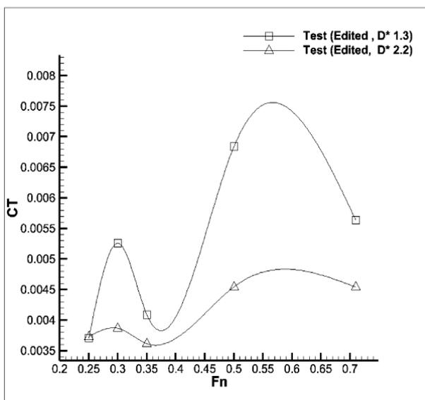
Fig. 3. The model resistance coefficient
