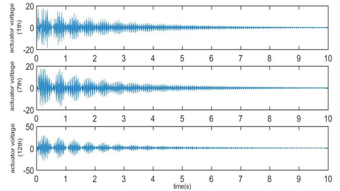
Figure 4. Voltage of first, seventh and twelfth actuator in terms of time.
