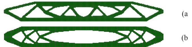
Fig. 3. Final topology of the 2 dimensional beam for maximum a) stiffness and b) fundamental frequency with 50% of volume fraction constraint.
