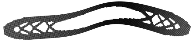
Fig. 2. Non-symmetric first mode shape in 27 th iteration
