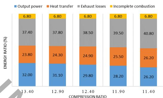
Fig. 5. Distribution of exergy ratio versus compression ratio
