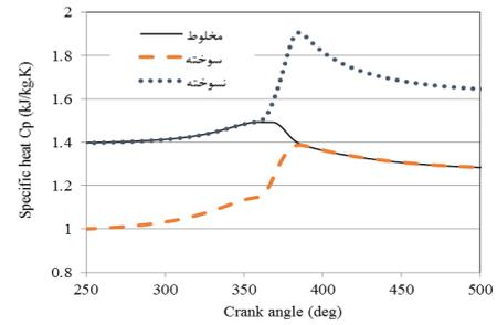
Fig.2. The specific heat of the operating fluid at constant pressure in terms of crank angle
