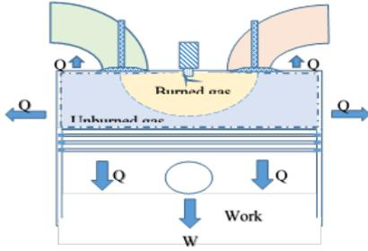
Fig. 1. The schematic view of the two-zone combustion model
