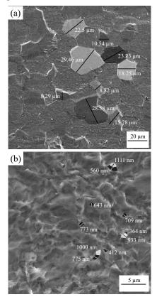
Fig. 4. Scanning electron micrographs of materials in (a) as recived condition and (b) after 4<sup>th</sup> pass of ECAP
