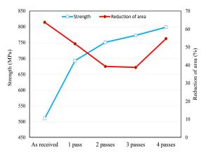
Fig. 3. Tensile strength and reduction of area for ECAPed samples at 260 °C
