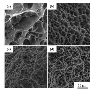
Fig. 5. fracture surface of (a) as recived material, and after (b) 1<sup>st</sup>, (c) 3<sup>rd</sup> and (d) 4<sup>th</sup> pass of ECAP
