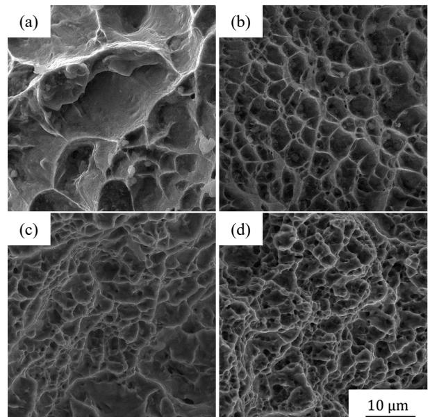
Fig. 5. fracture surface of (a) as received material, and after (b) 1<sup>st</sup>, (c) 3<sup>rd</sup> and (d) 4<sup>th</sup> pass of ECAP
