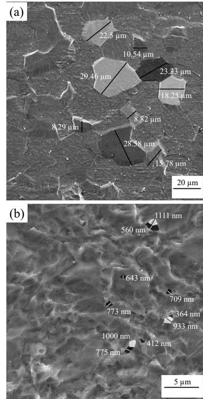
Fig. 4. Scanning electron micrographs of materials in (a) as received condition and (b) after 4<sup>th</sup> pass of ECAP
