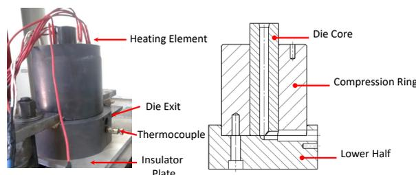
Fig. 1. ECAP die used in the experiments
