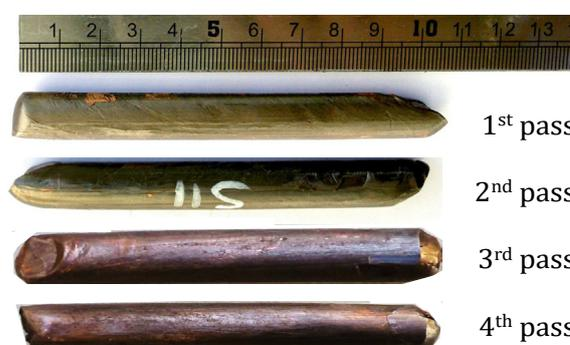
Fig. 2. Successful ECAP of grade-2 Ti at 260 °C
