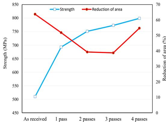
Fig. 3. Tensile strength and reduction of area for ECAPed samples at 260 °C
