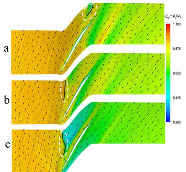
Fig. 4. Relative total pressure contour in span 0.97 with streamlines in three mass flow rates of (a) choke, (b) design and (c) near stall.
