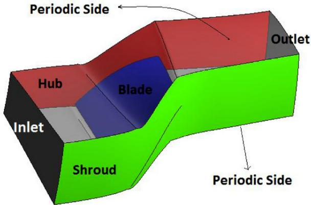
Fig. 1. Geometry and boundary conditions of NASA Rotor 37
