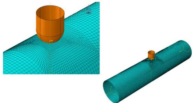
**Fig. 3: Modeling the impactor using analytical rigid shell and modeling composite cylinders using the S4R element**
