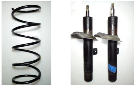
Fig. 2. Defected parts (spring and shock absorber) front wheel suspension
