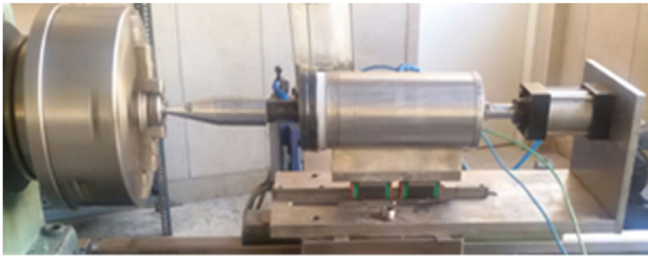
Fig. 2. Assembling of the UPT equipment on the lathe
