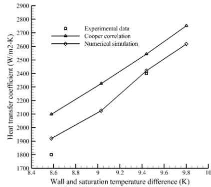
Figure 3. Heat transfer coefficient of experimental data [5], Cooper correlation [7] and numerical simulation
