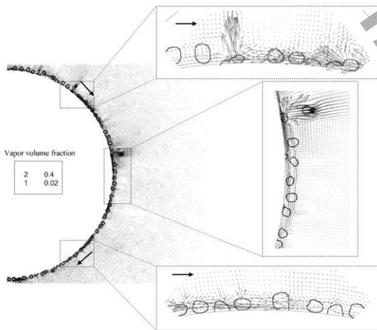
Figure 2. The influence of bubbles on the velocity vectors for the heat flux of  $18 \text{ kW/m}^2$  at 0.13 s
