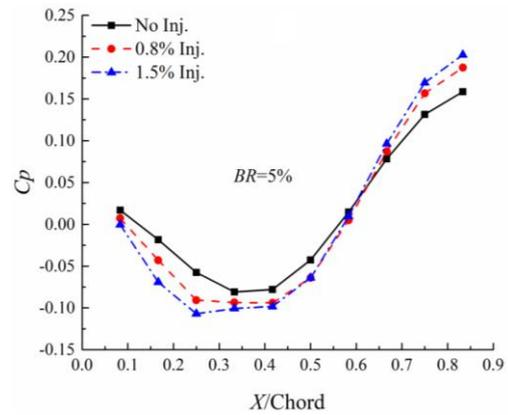
**Figure 3. Static pressure along the blade chord**
