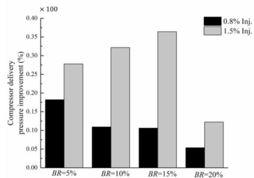
**Figure 4. Improvement of compressor delivery pressure**
