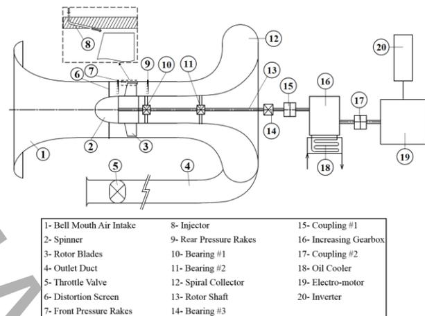
Figure 1. Schematic layout of IUST axial compressor test rig
