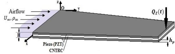
**Figure 1. The cantilever laminated CNTRC trapezoidal plate with two surface-bonded piezoelectric actuator layers subjected to a subsonic airflow and external transverse load.**
