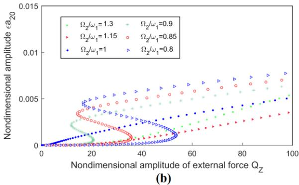
**Figure 3. Amplitude of response of (a) mode (1, 1), (b) mode (2, 2), versus amplitude of the external excitation for several frequency ratios in the presence of aerodynamic load, parametric excitation**
