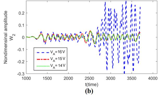
**Figure 4. Effect of the amplitude of electrical excitation on time response of (a) mode (1, 1), (b) mode (2, 2).**
