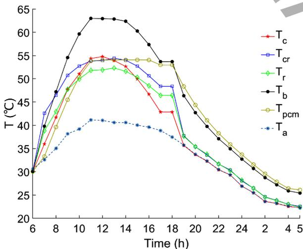
Fig. 4 Diagram of simulated temperatures of different components of the greenhouse solar dryer
