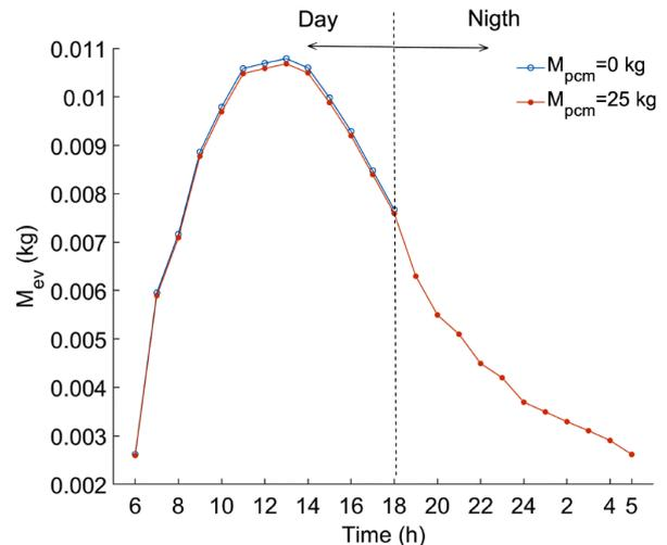
Fig. 5 Evaporation mass of the moisture in greenhouse dryer affected by presence and lack of PCM
