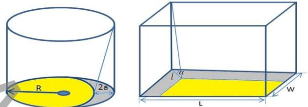
**Figure 1: Schematic of ponds with circular and rectangular cross sections along with their shaded areas**
