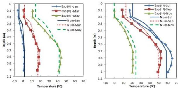
Figure 4: Temperature distribution predicted by numerical simulation with measured data for cubic pond of Urmia
