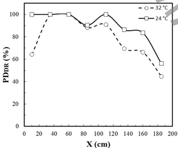
**Figure 3. PDDr changes along with the under-desk air diffusers' centerline**
