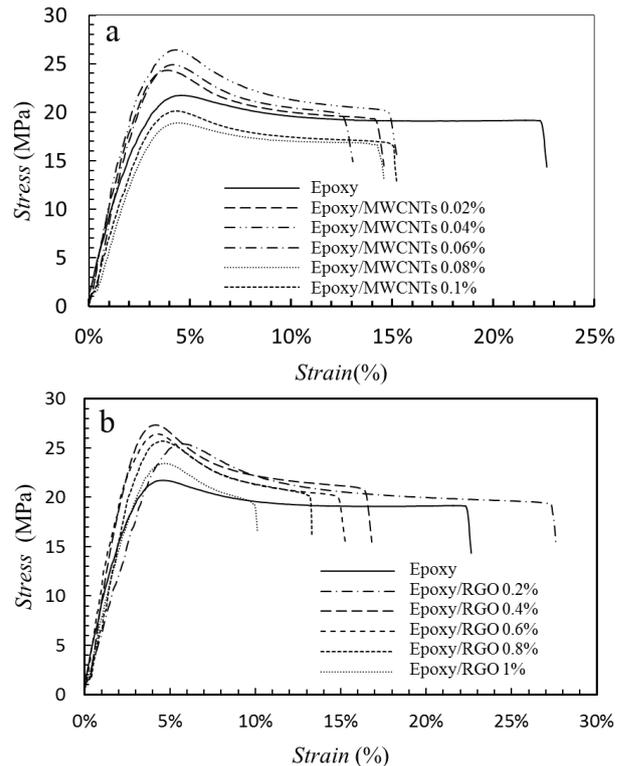
**Figure. 1 Strain-stress curve for a) Nanocomposites with different wt% of MWCNTs b) Nanocomposites with different wt% of RGO**
