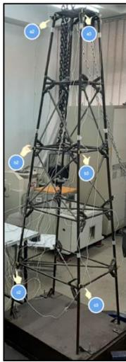
**Fig. 2. The laboratory offshore jacket model in intact state.**
