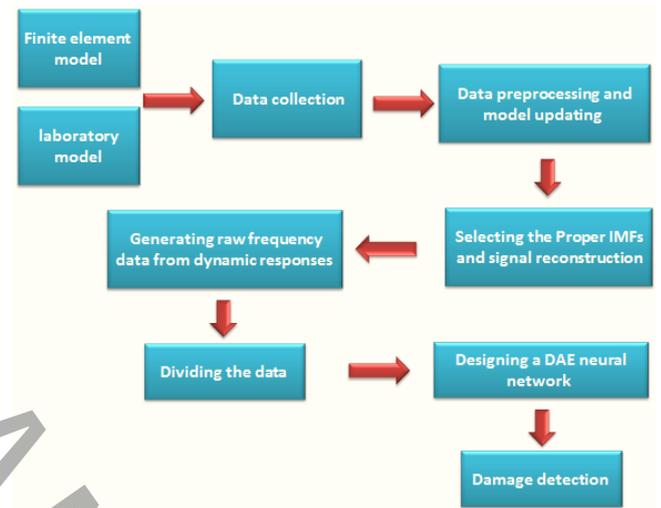
**Fig. 4. The block diagram of the proposed algorithm.**
