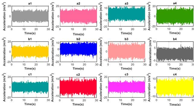
**Fig. 3. Extracted dynamic responses using 12 accelerometers mounted on the structure.**
