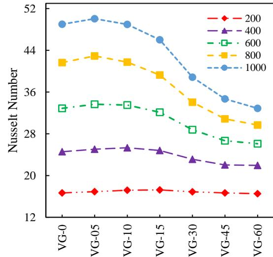
**Figure 3. Nusselt Number for all cases with vortex generator in different Reynolds numbers**
