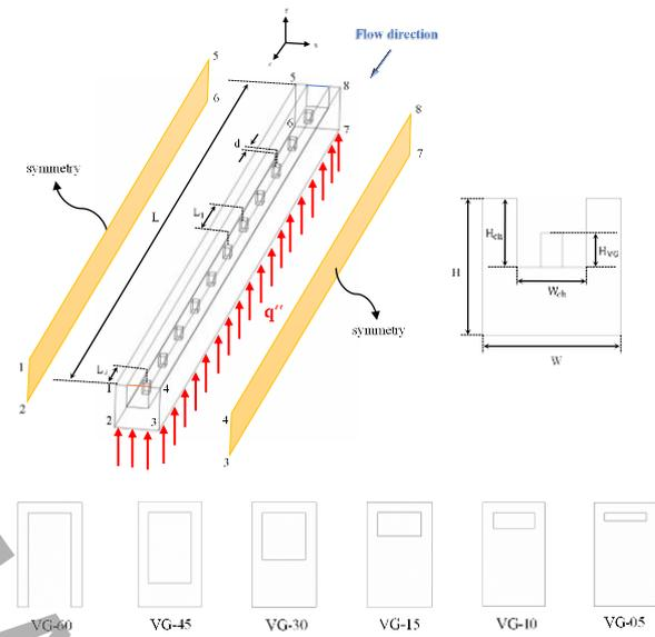
Figure 1. 3D view schematic of minichannel
