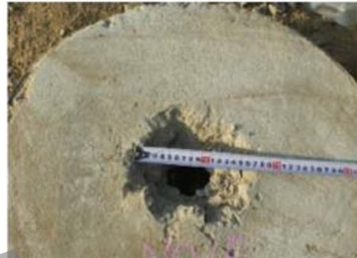
Fig. 2: Hole crater of the first target [3]
