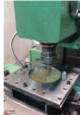
Figure 1. Performing the SPIF process on a CNC milling machine.
