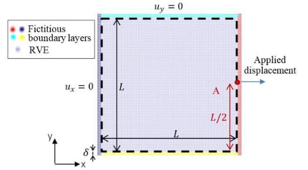
Fig. 2 Geometry of RVE and BCs
