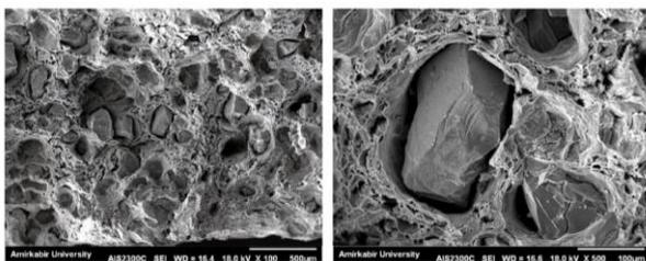
Fig.7. SEM images of the fractured specimens
