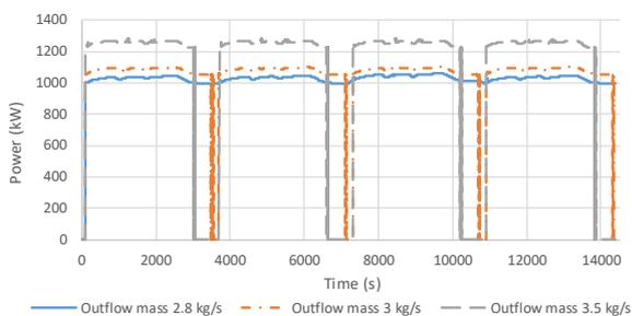
**Figure 2** The net power of ORC with different mass flow rate from steam accumulator
