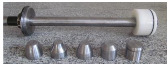
Fig. 1. The examined cushions (from right-to-left): cylindrical, conical, sagittal, parabolic and double conical.
