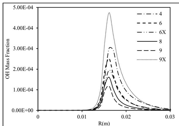
Fig. 5: Effect of co-flow pre-heating temperature on the  $\text{CO}_2$  injection in oxidizer on OH distribution
