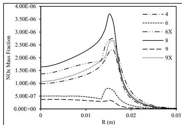
Fig. 6: Effect of coflow pre-heating temperature on the  $\text{CO}_2$  injection in oxidizer on NOx distribution
