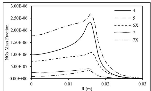
**Fig. 4: NOx distribution in 90 cm from inlets in different CO<sub>2</sub> mass fraction injection**
