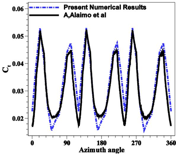
Fig. 3. Verification of straight-bladed turbine total moment coefficient
