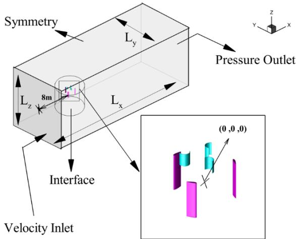
Fig. 2. The flow field and boundary conditions
