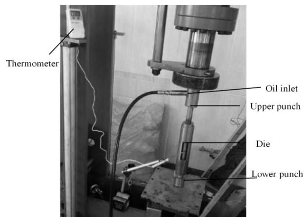
Fig. 1. Die set components mounted on the testing machine
