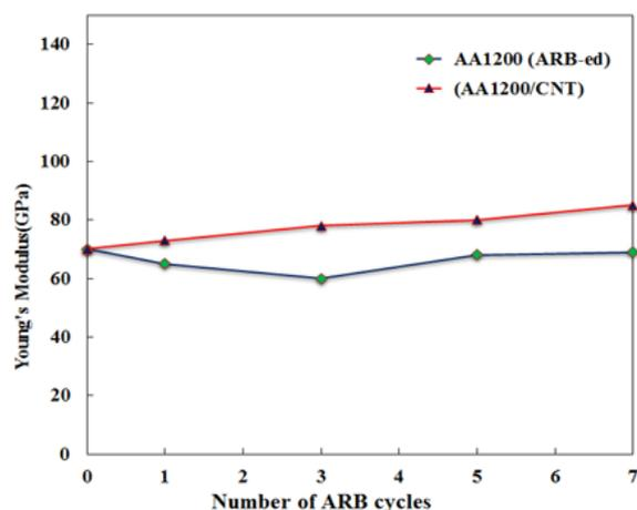
Fig. 5. The young's modulus variation of composite sheets AA1200 / CNT in different cycles of cumulative rolling process
