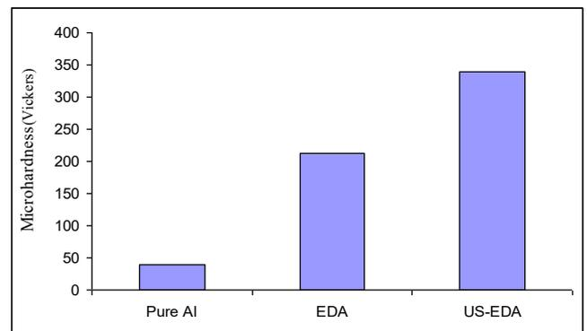
**Fig. 3. Effects of ultrasonic vibrations on surface hardness**
